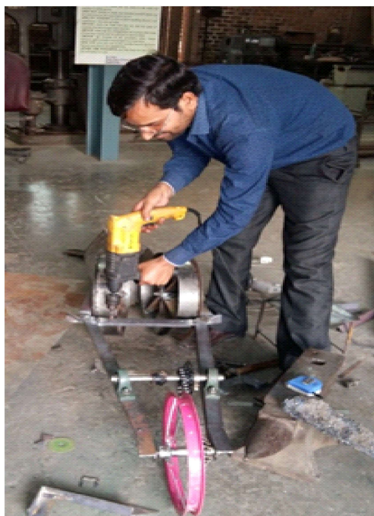
Plate 1. Fabrication process of manual operated single row planter for groundnut seed
