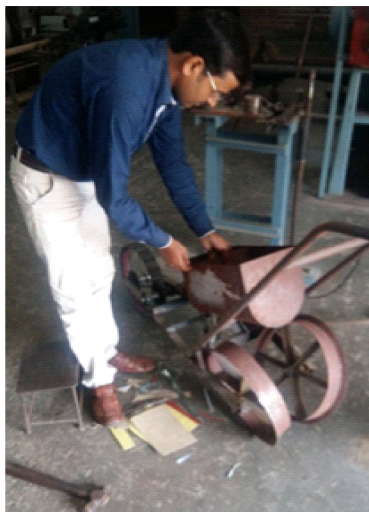
Plate 1. Fabrication process of manual operated single row planter for groundnut seed
