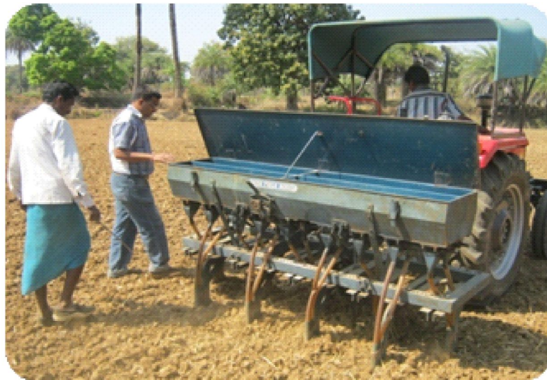
Plate 2. Sowing green gram in field using seed cum fertilizer seed cum fertilizer drill
