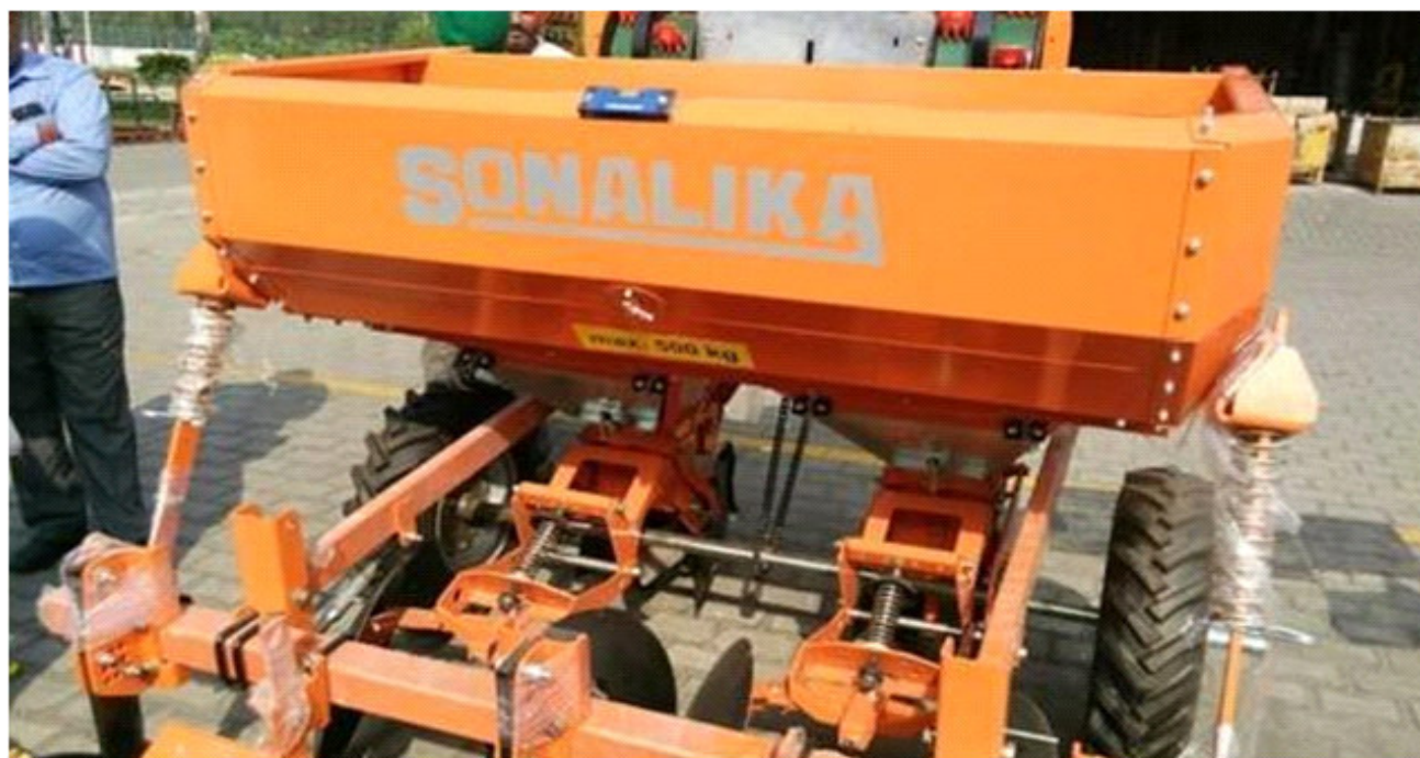
Fig 2. Automatic potato planter
