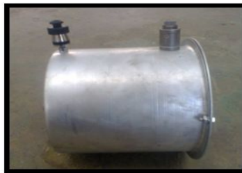
Fig 3. Hot air unit
