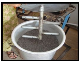
Fig 2. Arrangement of baffles inside the cylindrical drum
