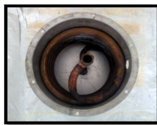
Fig 4. Copper coil fixed in the aluminium container
